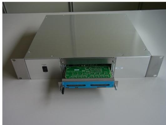
Figure 4: Digital controller board and the power supply box.
