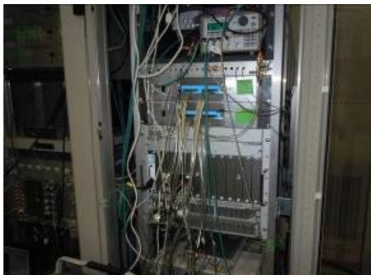
Figure 6: Test bench for digital controller board.
