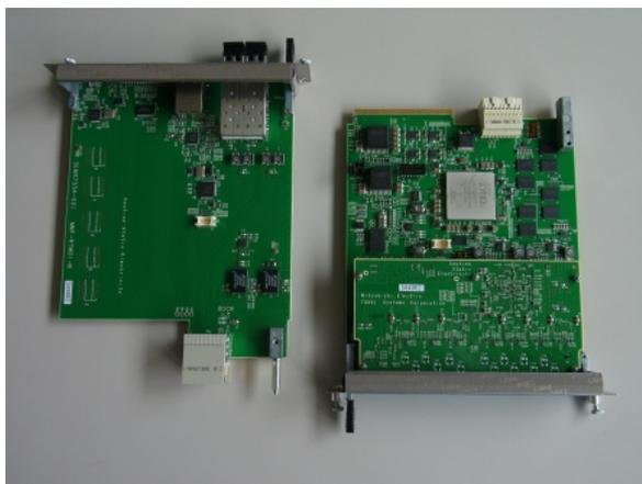
Figure 3: Digital controller board.
