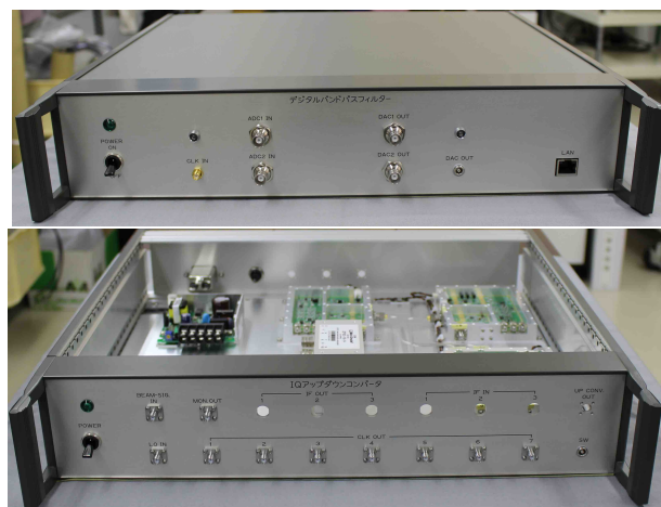
Figure 5: New damper for SuperKEKB (Upper: DF and lower: SSBF). Manufactured by Sanko-sha [6].
