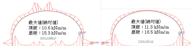
Figure 12: Maximum Moments (kNm/m, Left: with shielding wall, Right: no wall).
