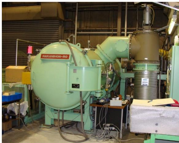
Figure 1: A furnace for 9-cell cavities, which were used for Nitrogen-doping.
