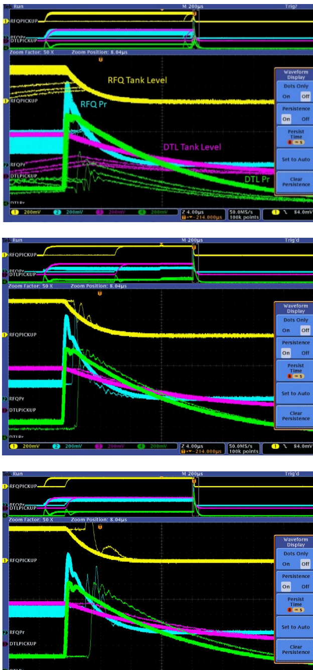
Figure 6: Aberrant waveforms remained today. The yellow shows tank level of RFQ. The cyan shows reversed RF power (Pr) from RFQ. The magenta shows DTL tank level. The yellow-green shows Pr from DTL.
