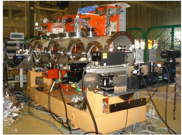
Figure 4: Prototype A (left) and B (right) of lightweight compact IVU based on force cancellation system using MMMs [1].
