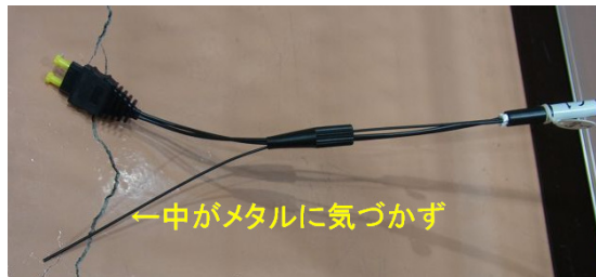
Figure 4: Discharged with this optical fiber cable
