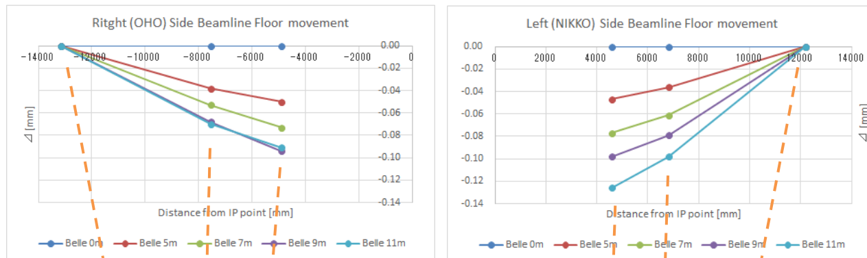
Figure 9: Beamline floor movement.
