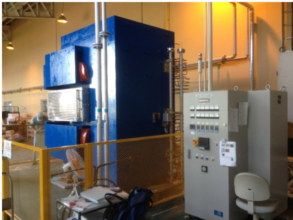
Figure 1: Magnetic annealing oven for the mass production.
