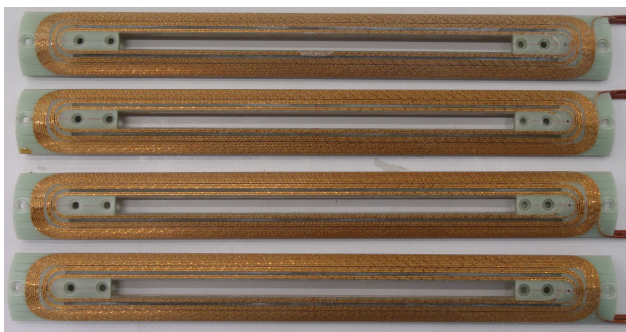
Figure 5: 4 SC coils for QC1LP magnet.
