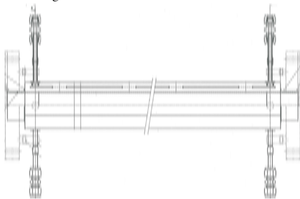
Figure 1: Structure of the ceramic chamber of HER Injection kicker.
