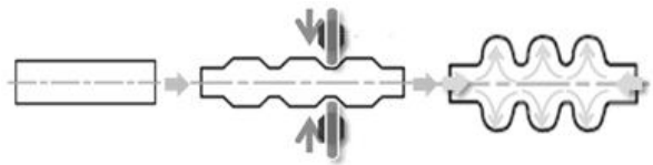
Figure 4: Manufacturing flow of seamless cavity.
