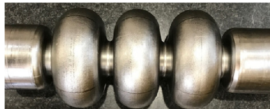
Figure 5: 3-cell seamless cavity.
