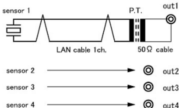
Figure 2: Circuit diagram of acoustic sensor.
