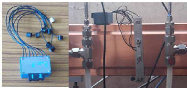
Figure 3: Acoustic sensor & attach to the load.
