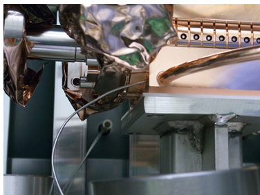
Figure 3: Copper foil shield in the vicinity of coupler wave guide opening during K2 vacuum baking.
