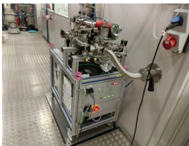
Figure 12: Picture of slow pumping system for EURO-XFEL.
