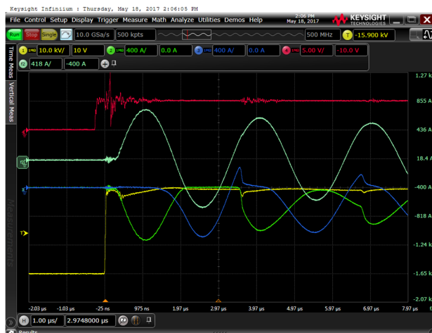
Figure 2: Typical waveform with the switch of high withstanding voltage configuration (wavefront). Traces are same as those shown in Figure 1.
