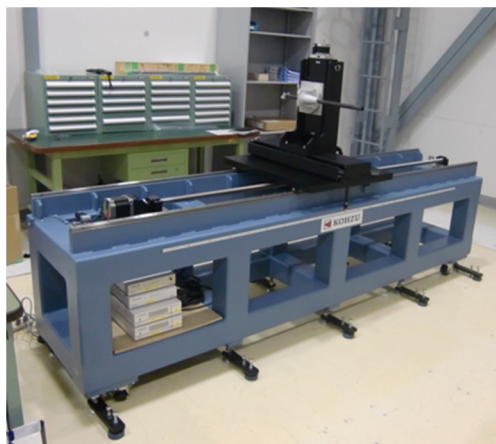
Figure 5: Three-dimensional magnetic field measurement system.
