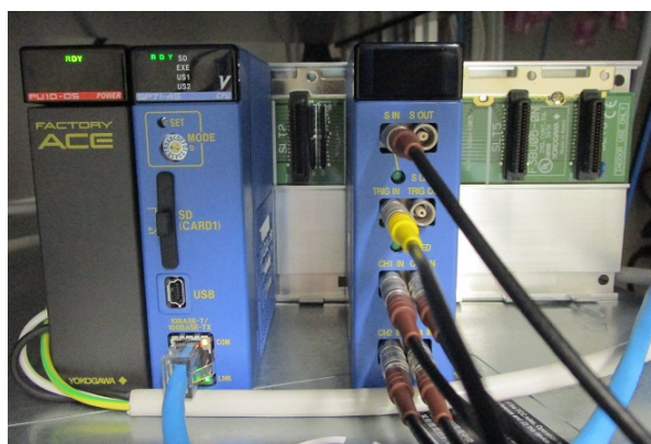
Figure 7: A picture of test set for a triggered scaler.
