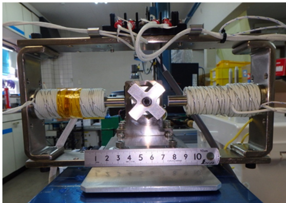
Figure 6: Photograph of a prototype of the rotation sensor with a 4-poles rotor. A gap between the pole and the rotor is 0.5 mm. The right side is the excitation coil, and the left side is the pickup coil.
