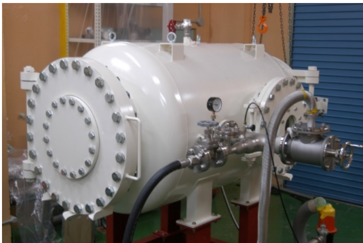
SF6 insulator gas tank
