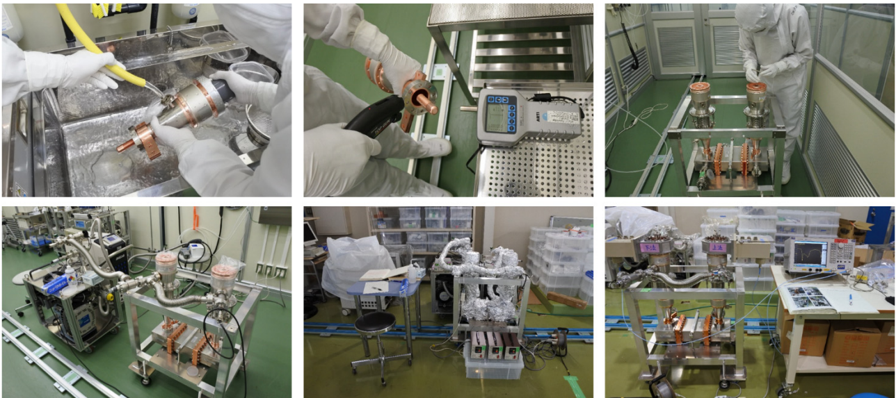
Figure 3: Status of the assembly work in the clean room, the baking, and the low power test by the network analyser. From left to right in the top figures: the ultrapure water rinsing, cleaning by the ion gun, and jointing between the warm and cold parts. From left to right in the bottom figures: the pumping and the leak check, the baking, and the low power test.
