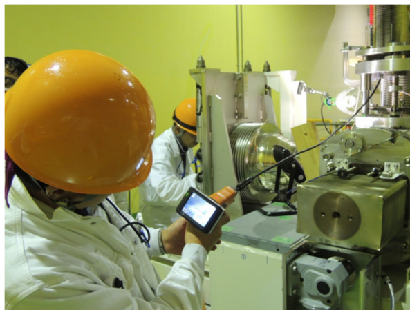
Figure 6: The aspect of a work to specify vacuum leakage point.
