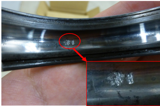
Figure 6: Scratches on bearing.
