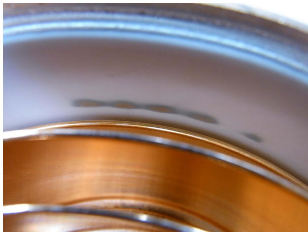
Figure 5: Discharge trace on ceramic surface.
