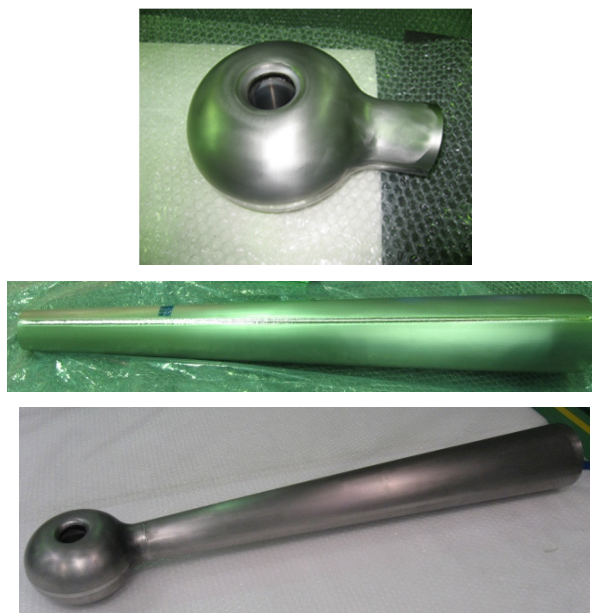
Figure 2: drift tube (top), stem (middle) and sub-assy (bottom).
