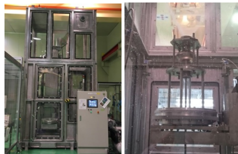
Figure 6: High pressure rinse facility.
