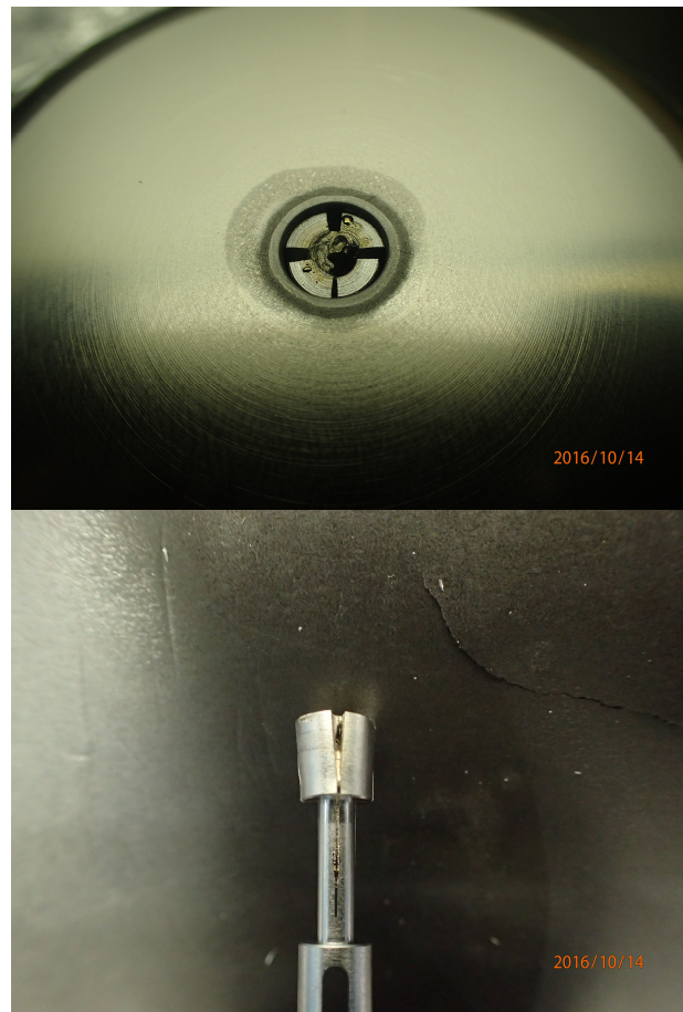
Figure 4: Melted CeB 6 cathode with the molybdenum sleeve.
