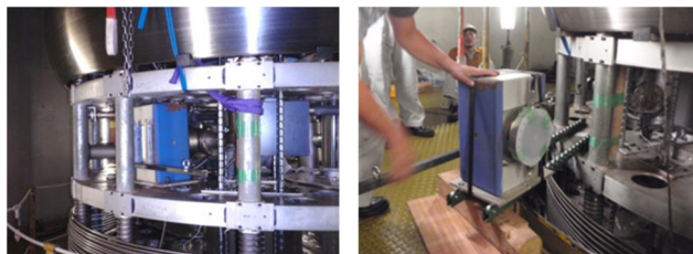
Figure 11: Removal of ion pump from dead section.
