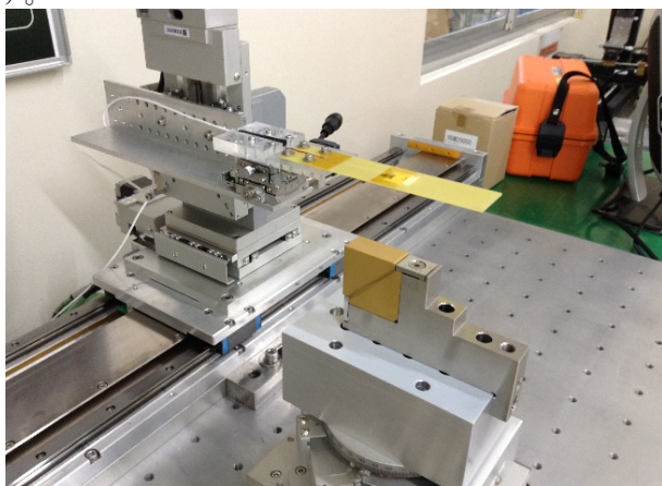
Figure 3: Measurement setup for individual magnetic blocks along the beam axis using two-dimensional Hall probes system. The height of the probes above the magnet surface is 12 mm, corresponding to a minimum gap of 24 mm.
