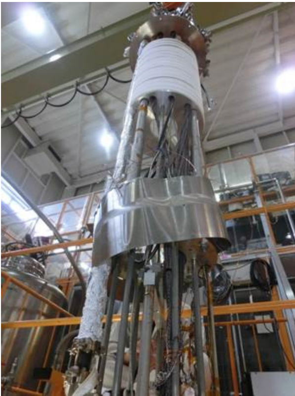
Figure 12: Broken magnetic shield wrapped around the cavity hanging parts.
