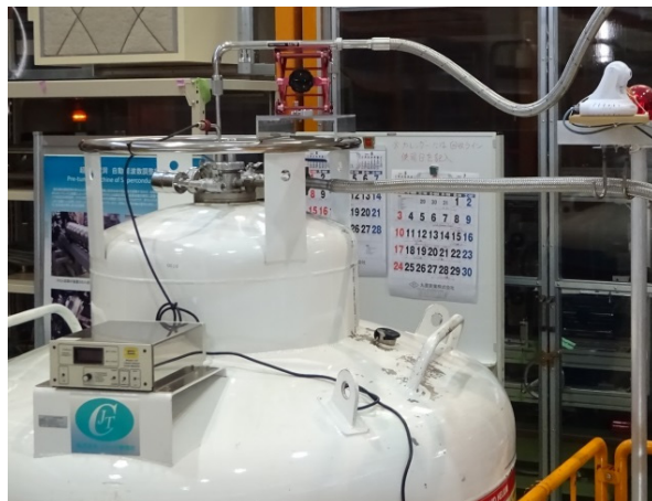
Figure 10: Transfer tube line after insertion into helium dewar.
