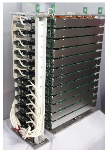
Figure 3: Appearance of the 50 kV solid-state switch.
