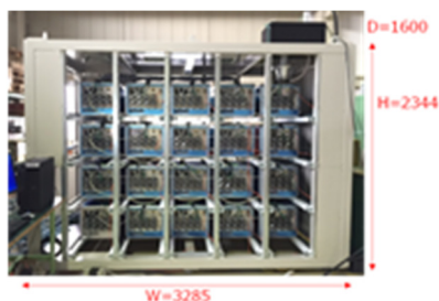
Figure 2: SiC MOS FET MARX power supply for ILC klystron modulator.
