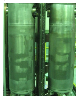
Figure 8: Welding of cavities.
