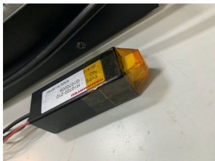
Figure 3: Photograph of the detector constituted with a CsI(Tl) scintillator and a photomultiplier-tube.
