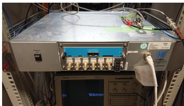
Figure 1: LLRF box. The BNC connectors in the front panel are auxiliary inputs to the RTM.
