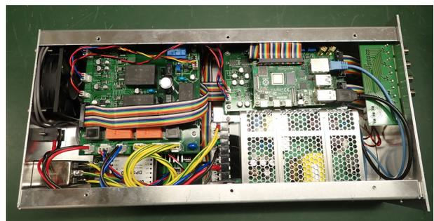
Figure 1: Magnet Power Supply.
