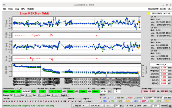
Figure 1: Beam orbit panel developed by Python/Tkinter.
