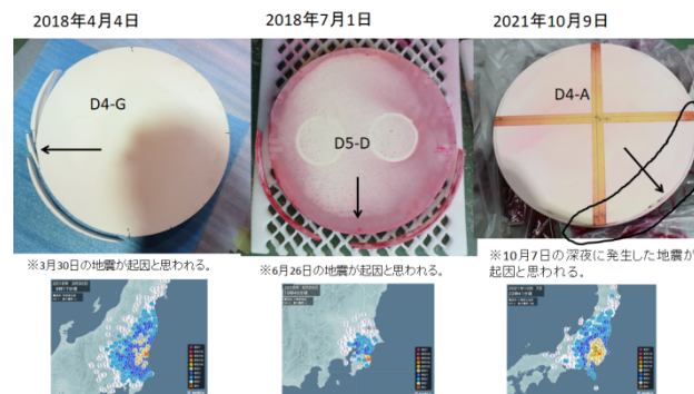
Figure 5: Broken RF window with water leak.
