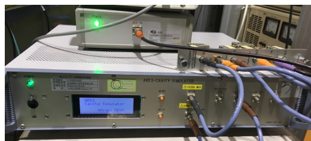
Figure 5: Photo of the ARES cavity simulator including piezo tuner function.
