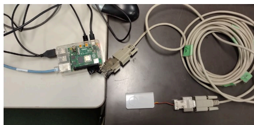
Figure 1: Real-time monitoring system using a portable radiation counter and Raspberry Pi, which are connected through a Dsub cable.
