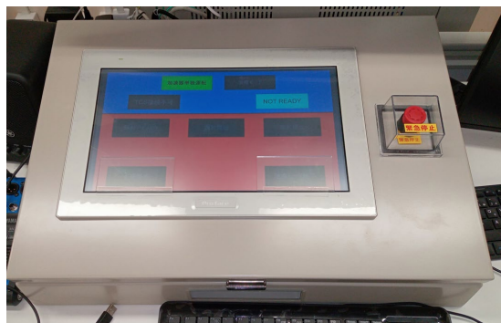
Figure 3: Photograph of a developed doctor-operated control panel which equips a touch panel and an emergency stop button to stop irradiation.
