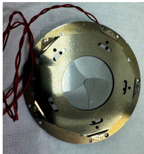
Figure 3: View of the target with the shutter portion modified with a titanium blade.
