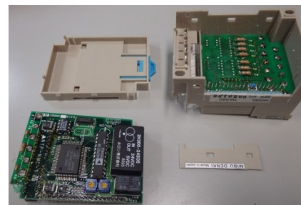
Figure 5: Remove the substrate with DC-DC converter and transceiver IC from the frame body.
