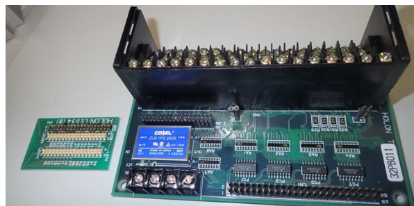
(c)After removing LED board, converter appears.
