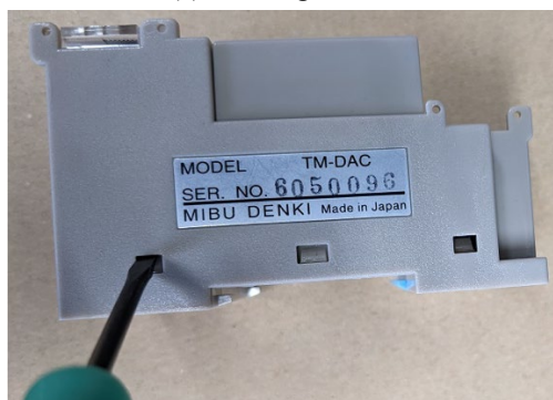
(b) push the crawls and lever open the cover.
