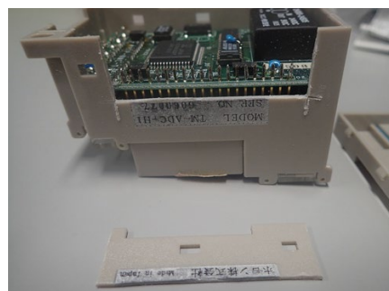
(a) Cut a part of frame body near 22 pin header.
