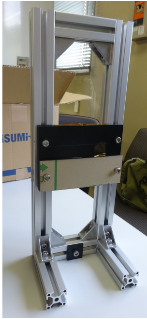
Figure 3: Overall view of a jig for irradiating films and dosimeters. The contents of the black acrylic plate in the middle are shown in Fig. 2.
