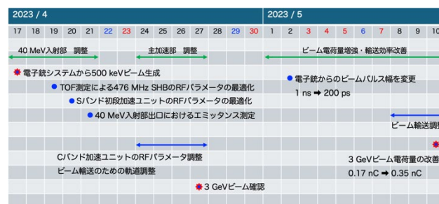
Figure 4: Timeline of beam commissioning 3-GeV linear accelerator.
