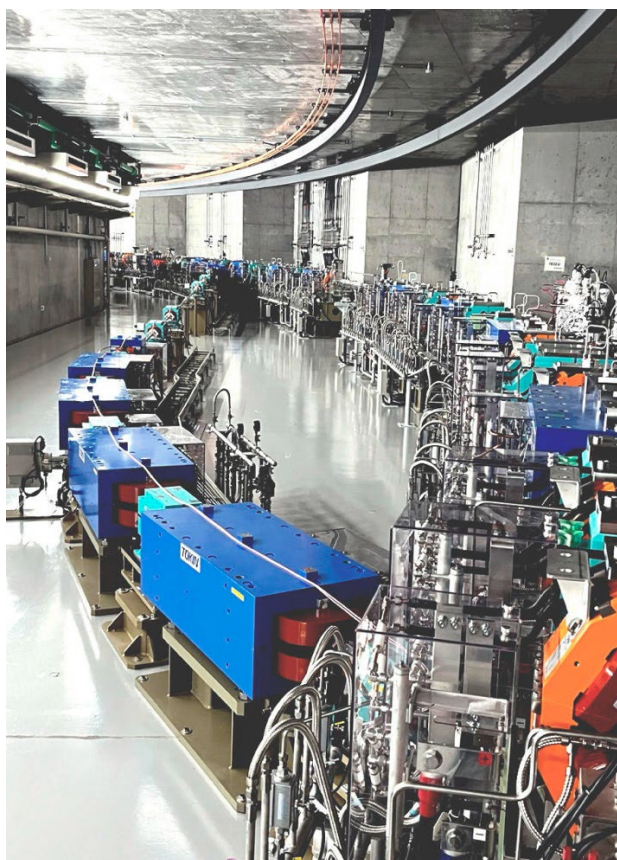
Figure 3: Photograph of 3-GeV beam transport line and injection point of storage ring.
