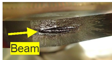
Figure 2: Collimator head damaged by SBL.
