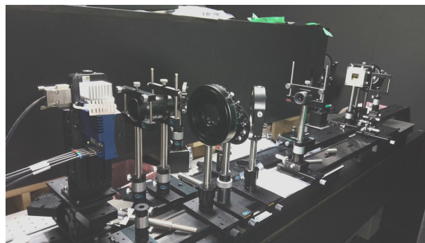
Figure 4: Gregorian telescope and ultrafast CMOS camera.
