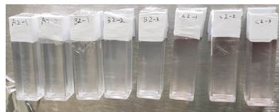
Figure 3: PVA-I gel dosimeter placement. An example of setting of II in Figure 2 is shown. The left side (A side) is the beam entrance side, and the right side (C side) is the outside of the undulator. The same placement was used for all locations.
