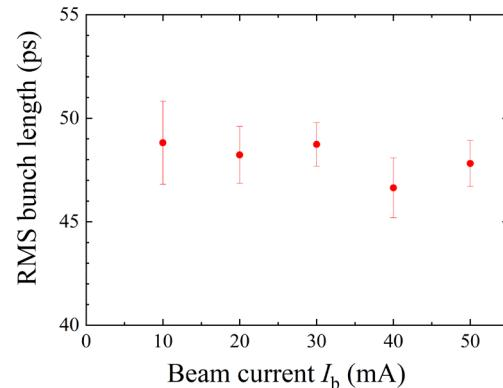
Figure 6: Measured rms bunch length as a function of the beam current. Beam energy:  $6.5 \text{ GeV}$ .
