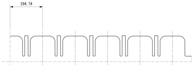
Figure 8: Inner shape of the APS cavity. Only upper half of the cavity is shown.
