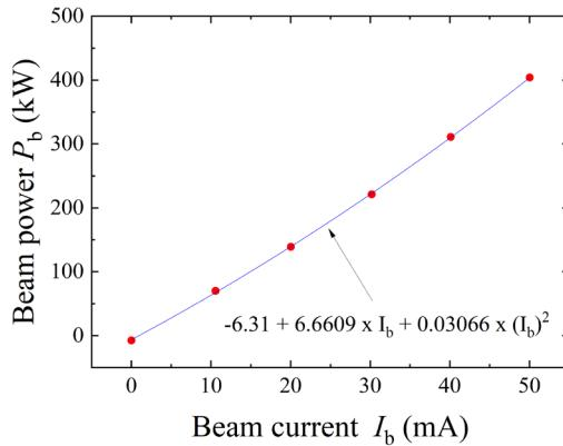
Figure 4: Beam power ( $P_b$ ) as a function of the beam current at  $6.5 \text{ GeV}$ . Solid line denotes the fitting result.
