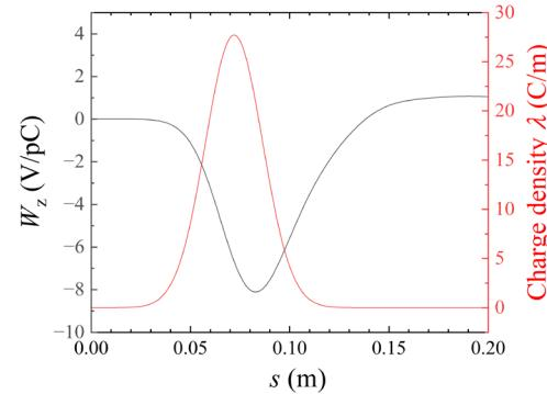
Figure 9: Calculated longitudinal wake potential (black line) of the APS cavity for a bunch length of 14.4 mm. Assumed charge distribution is also indicated by red line.
