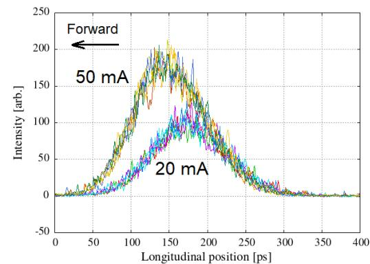
Figure 5: Longitudinal bunch profiles observed at beam currents of  $20 \text{ mA}$  and  $50 \text{ mA}$ . For each beam current, five traces were overlaid. Beam energy:  $6.5 \text{ GeV}$ .
