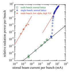
Figure 1; CSR power vs. stored beam current per bunch. Square: case (A); normal  $\alpha$  with multi-bunch, diamond: case (B); normal  $\alpha$  with single bunch, triangle: case (C); low  $\alpha$  with multi-bunch.
