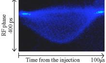
Figure 8; Change of the length of the injected bunch in the storage ring. The left end is the injection timing [18].
