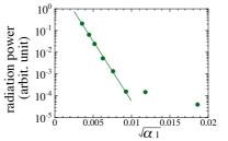
Figure 4; CSR power dependence on the momentum compaction factor ( $\alpha_1$ ). Here  $V_{RF}$ =120kV.
