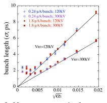
Figure 3; Momentum compaction factor  $\alpha$  vs. RMS bunch length measured by a streak camera.
