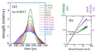
Figure 2; Beam current dependence of the longitudinal bunch shape. (a) shows the bunch shape normalized with the current and (b) shows the current dependence of the peak current and FWHM of the bunch.
