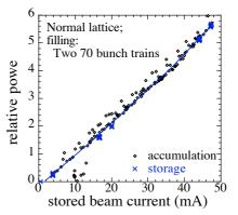
Figure 7; THz radiation power in normal condition, during the accumulation and the storage (no injection). Square data points above the line, on which the data points of the storage (cross) are, show the power rise by CSR from the linac beam.
