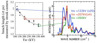
Figure 6; The dependence on the power spectrum on the bunch length. (a) shows the bunch compression by  $V_{RF}$ . (b) shows the power spectrum at three settings of  $V_{RF}$ .
