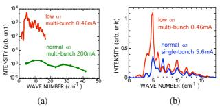
Figure 5; Radiation power spectrum from the stored beam. (a) shows those in condition (A): normal incoherent radiation and in condition (C): steady state CSR. (b) shows those in condition (B): CSR burst, and that in condition (C)
