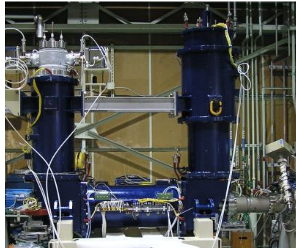
Figure 1: Picture of the constructed compact electron cooler. The cooling solenoid length is 0.8 m the magnetic field 0.5 kG and the maximum expansion factor is 3.
